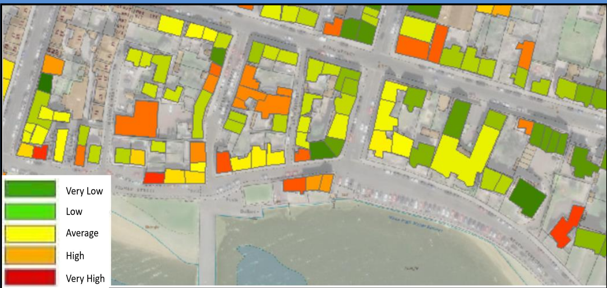
Figure 2: Section of a vulnerability map for Broughty Ferry under an extreme 7m inundation Scenario
